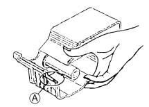
1. Open the right cover. Then push the head-up lever in the direction indicated by the arrow.
